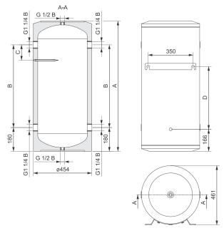
Connection and installation dimensions of the wall-mounted version of the buffer tank (mm)
