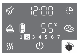
Figure 13: Example of setting the timer – radiator heating
